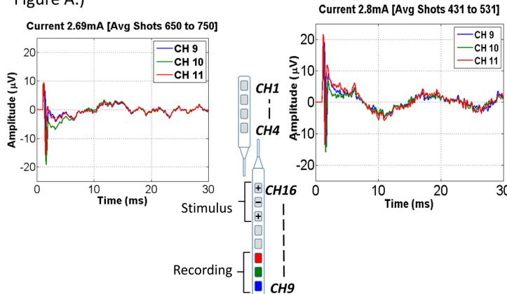
**Figure A. Recordings after stimulation on the S8 Lamitrode™, during procedure (left) and at closing (right). Signals are ECAPs propagating from CH11 to CH9**
