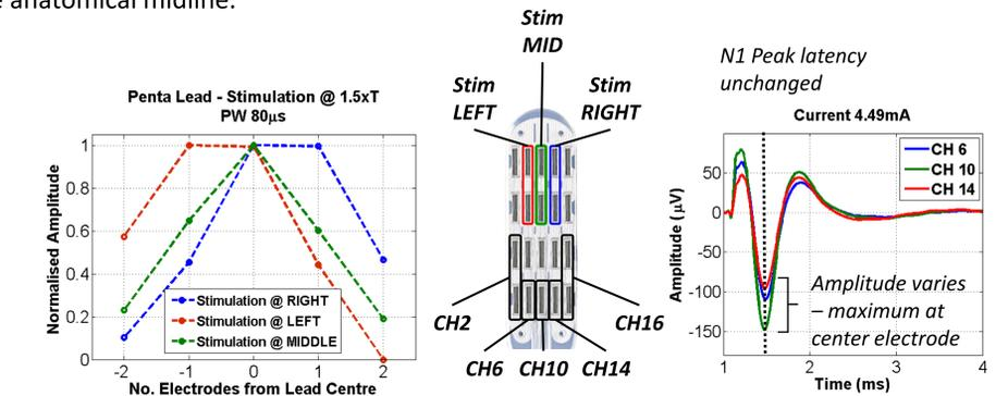
**Figure C. ECAP Amplitude correlates with lateral distance from the stimulating electrode, on both sides (left). ECAP latency does not vary with the lateral distance from the stimulating electrode (right).**
